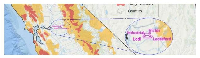
Note: Three 60kV transmission lines originating from PG&E's Lockeford substation, operated and maintained by PG&E, enter LEU's service territory at the Industrial substation.
