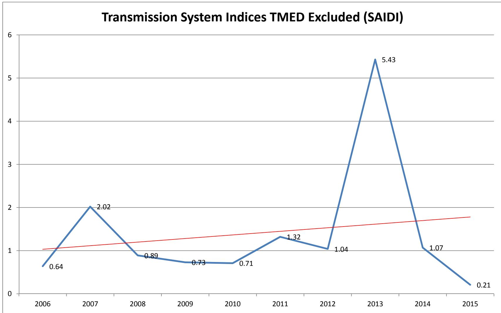
Note: The peak in 2013 is due to the Borrego Outages. Outage events were caused by extreme weather such as high winds and rain storms
