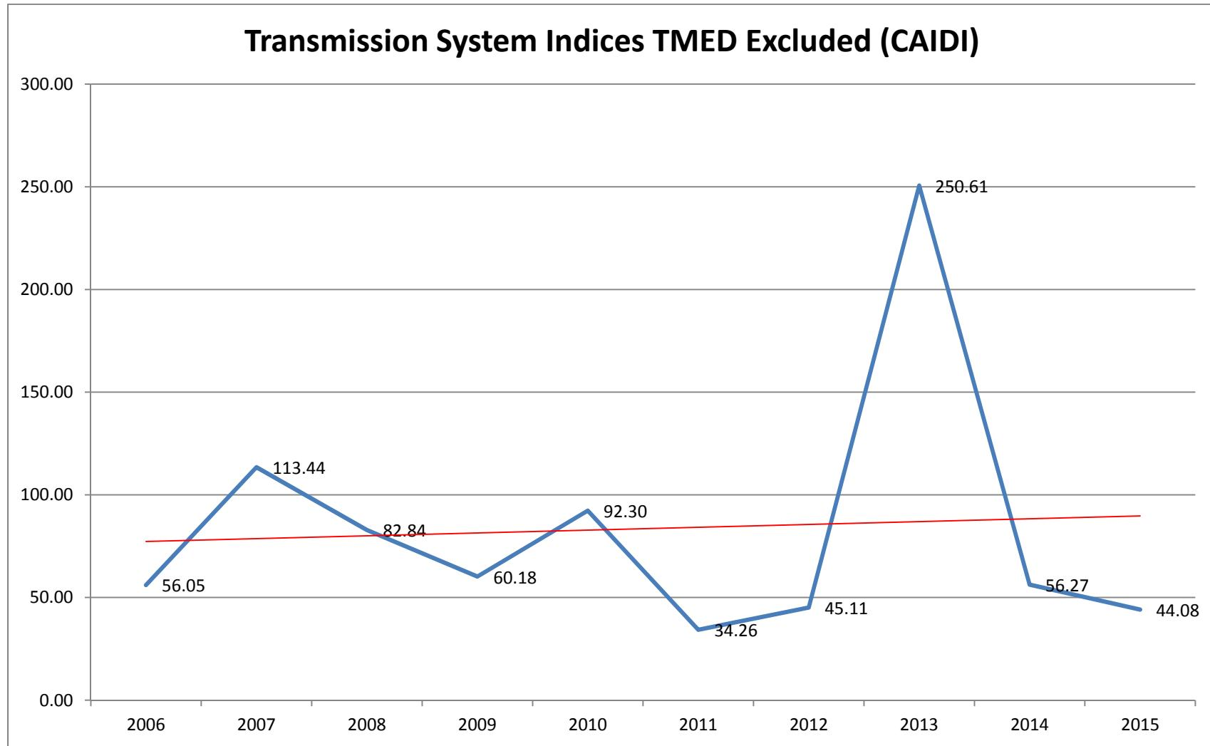
Note: The peak in 2013 is due to the Borrego Outages. Outage events were caused by extreme weather such as high winds and rain storms
