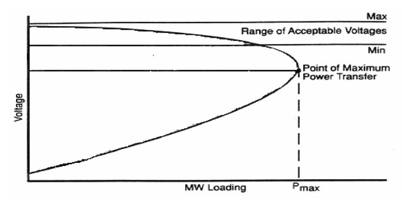
P-V analysis (real power relative to voltage) is a tool which determines the real power transfer capability across a transmission interface for load supply.
