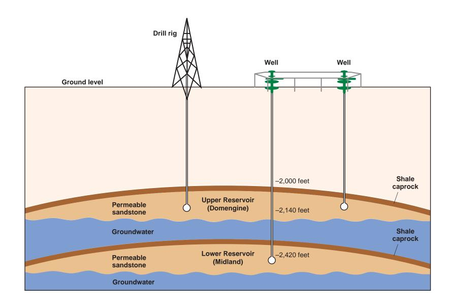
Figure ES-2 Conceptual Cross-Section of Lodi Gas Storage Field
