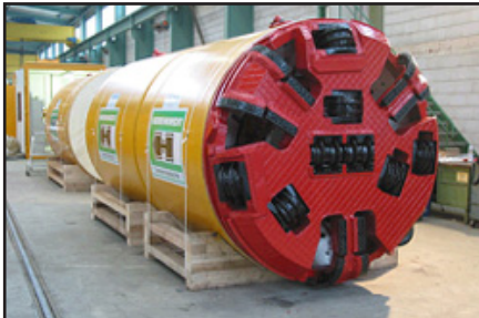
Microtunnel Boring Machine
