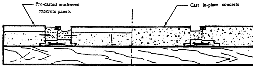
TYPICAL CROSS SECTION
