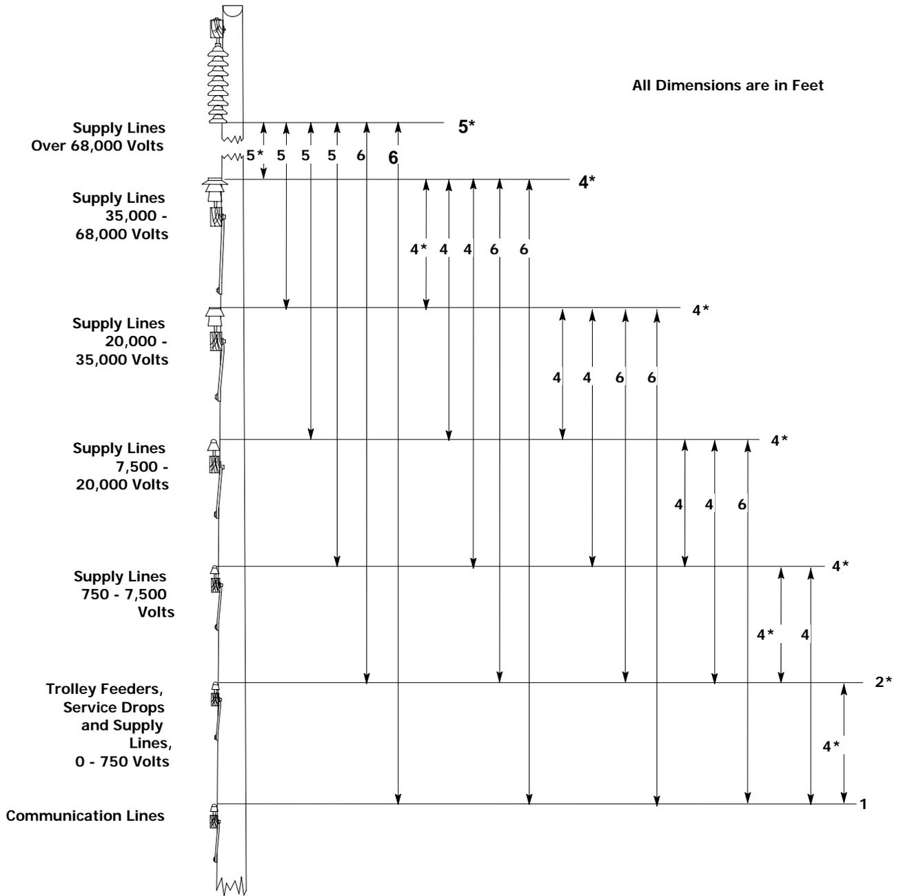
Note: Figure at extreme right of each conductor level is the separation between conductors of same voltage classification
