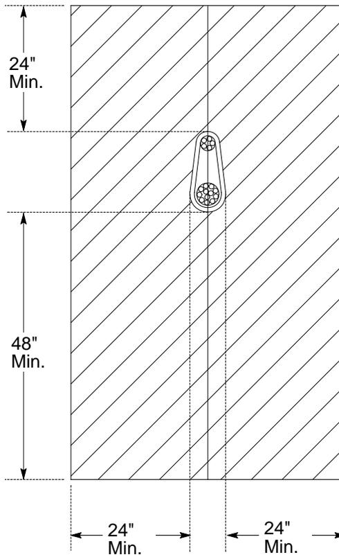
Note: No supply service drop within shaded area see Rule 57.4 for method of measurement
