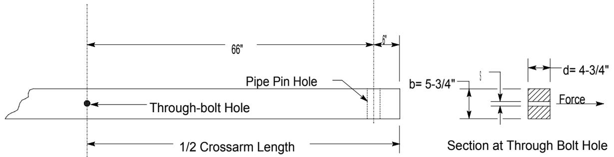
The section through the arm and the method of computing the fiber stress is shown below.
