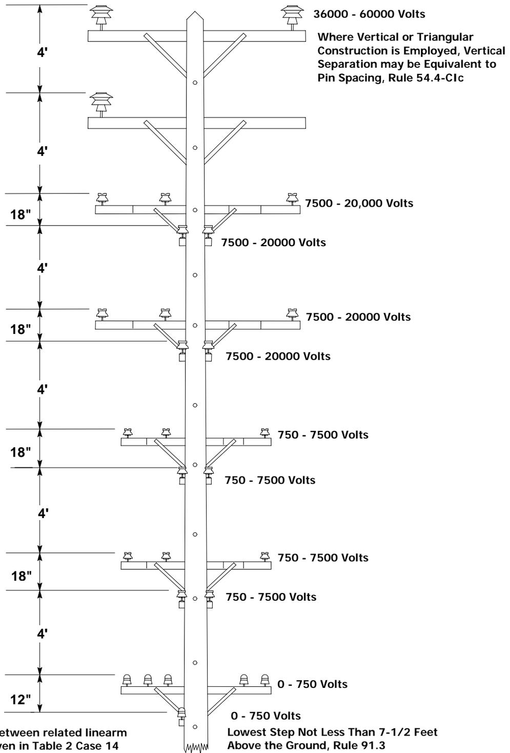
Note: Clearances between related linearm and buckarm as given in Table 2 Case 14 shall not be applied consecutively both above and below the same conductor Rule 54.4-C2
