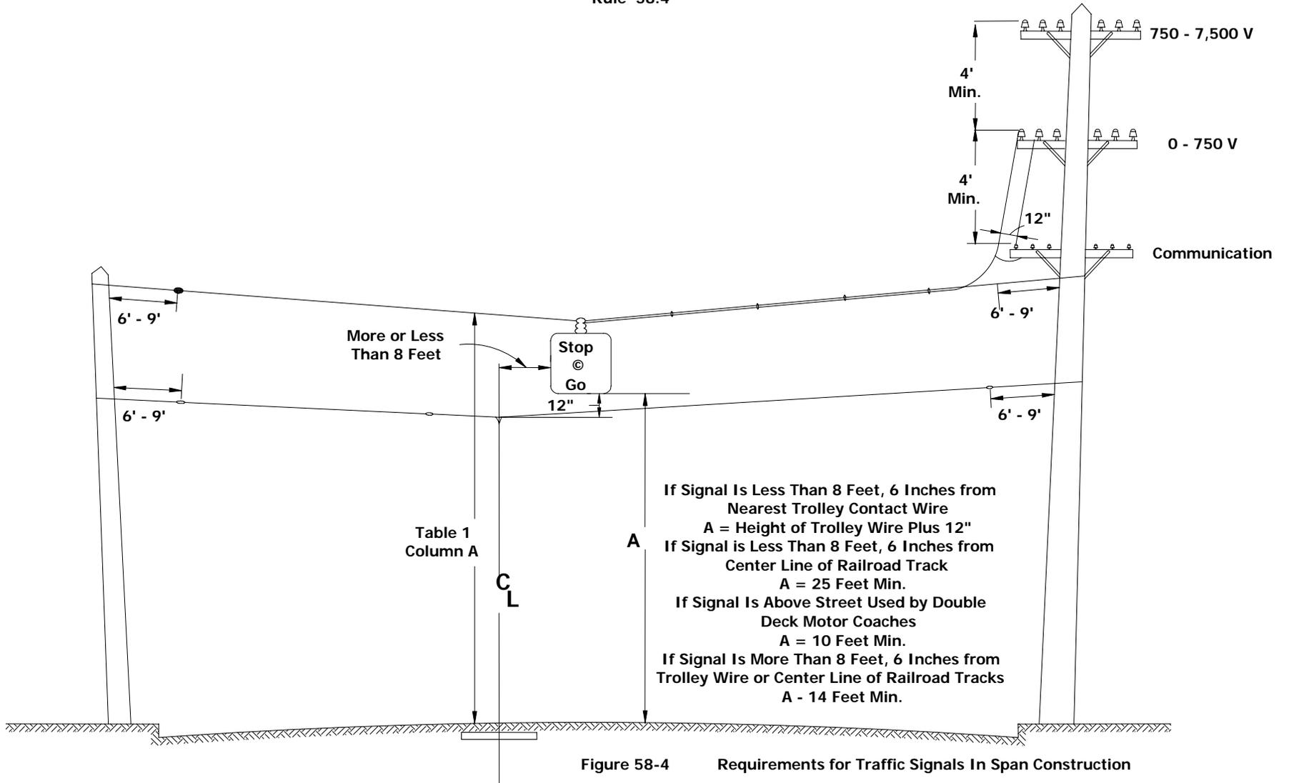
Figure 58-4 Requirements for Traffic Signals In Span Construction
