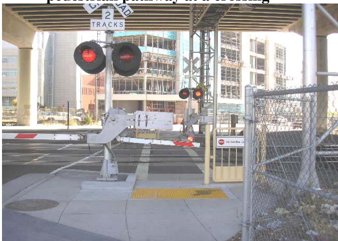
Figure 13. Detectable warning surface across pedestrian pathway at a crossing
