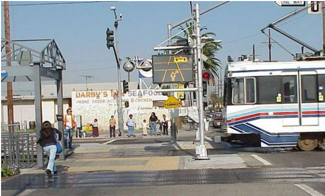
Figure 42. Sign indicates an approaching train
