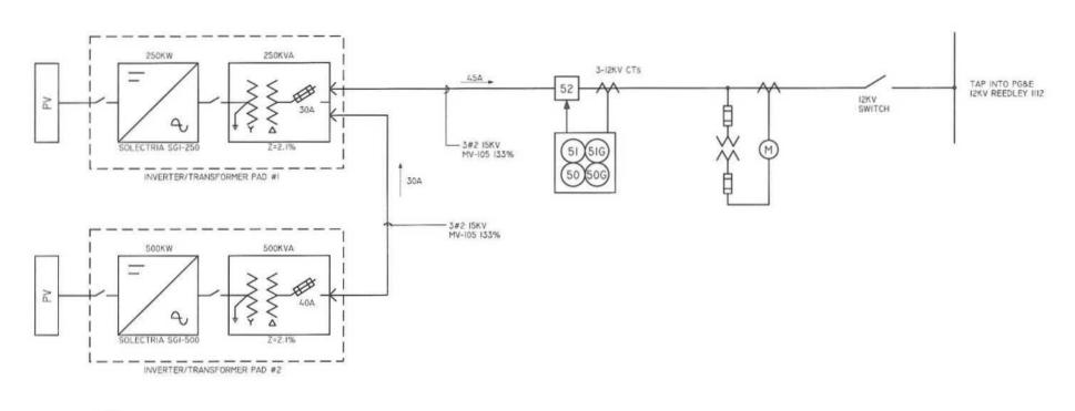
NOTE: PV MODULES AND INVERTERS ARE CEC LISTED. TOTAL SYSTEM SIZE = 750KW
