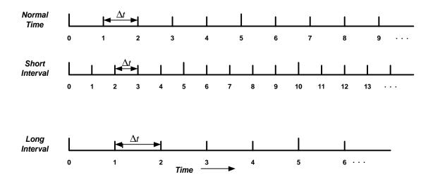
For each of the illustrations shown above, the actual interval of measurement is different. We assume that the meter and the computer systems are synchronized at some time,  $T_0$  {for example, the last meter read} and that the meter is now being read at a read time,  $T_r$ . For each case above, assume that the meter reading system reads at the same time. The elapsed time is given by
