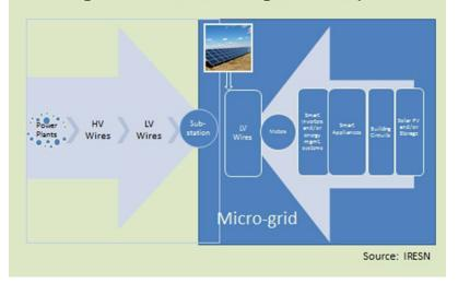
community based solar generation capacity in California suggests a likely prevalence of solar microgrids, shown conceptually in Figure 7<sup>15</sup>.
